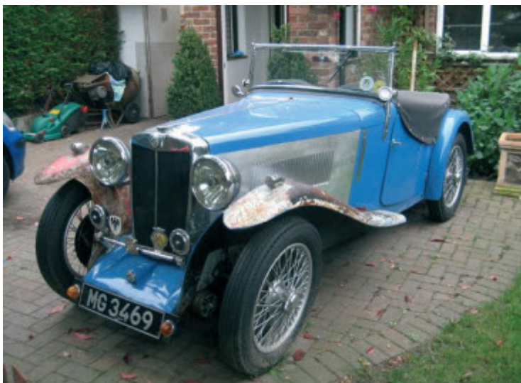
Malcolm Bailey's ND with its incorrect P-type wings awaiting its new ND wings at James Pettit's
